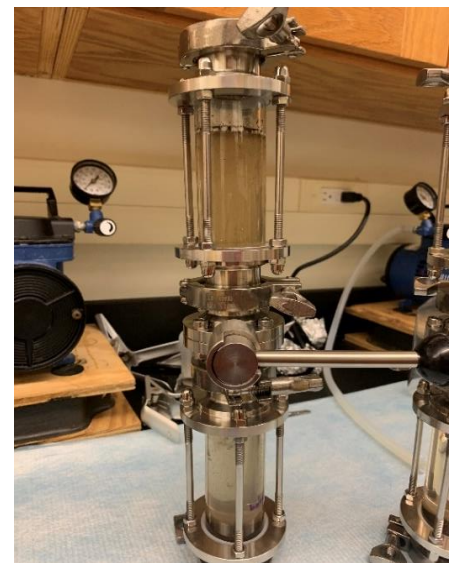
Figure 1. Density separation device (DSD) schematic (left) and during the lab separation(right) (after Löder et al., 2015).
