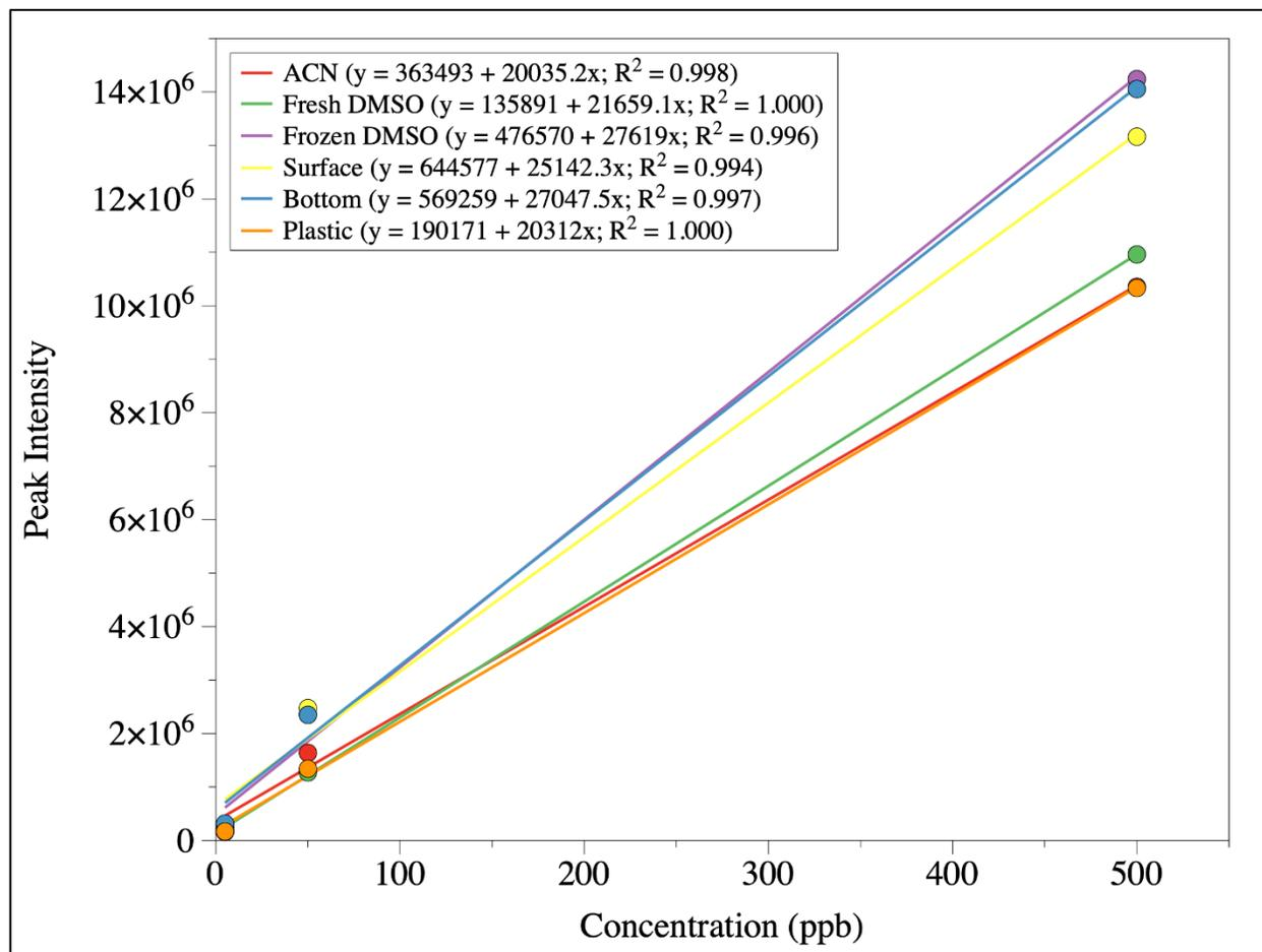
**Figure 4.** Effects of solvents and preparation approaches on the measurement of 6PPD-quinone.
