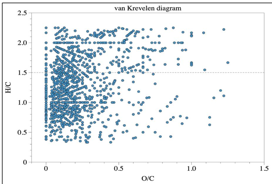
**Figure 3.** van Krevelen diagram of detected formulas in the tire particle leachate. Each dot represents a unique formula. A total of 1,368 formulas were calculated and assigned.
