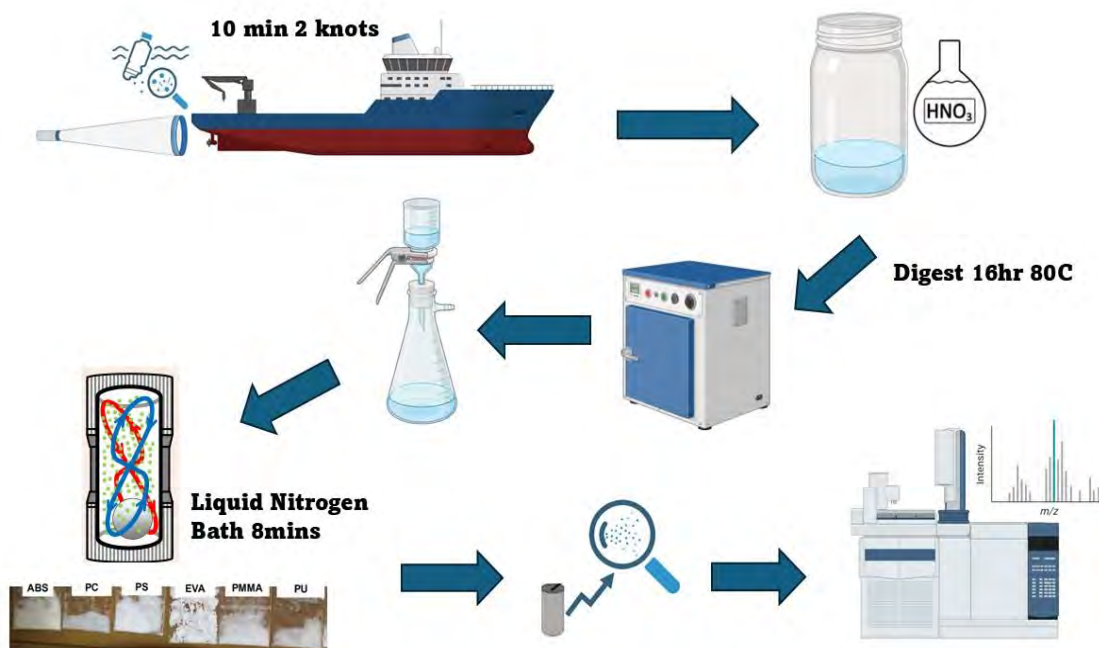
Figure 5. Graphical representation of sampling and analytical protocol of suspended microplastics. The plankton tow typically can filter 10-50k liters of seawater with a mesh size 150 \mu m. We used nitric acid with sodium persulfate to remove the natural organic matter, while the microplastics remain largely intact. After the cryogenic milling, a subsample can be analyzed
