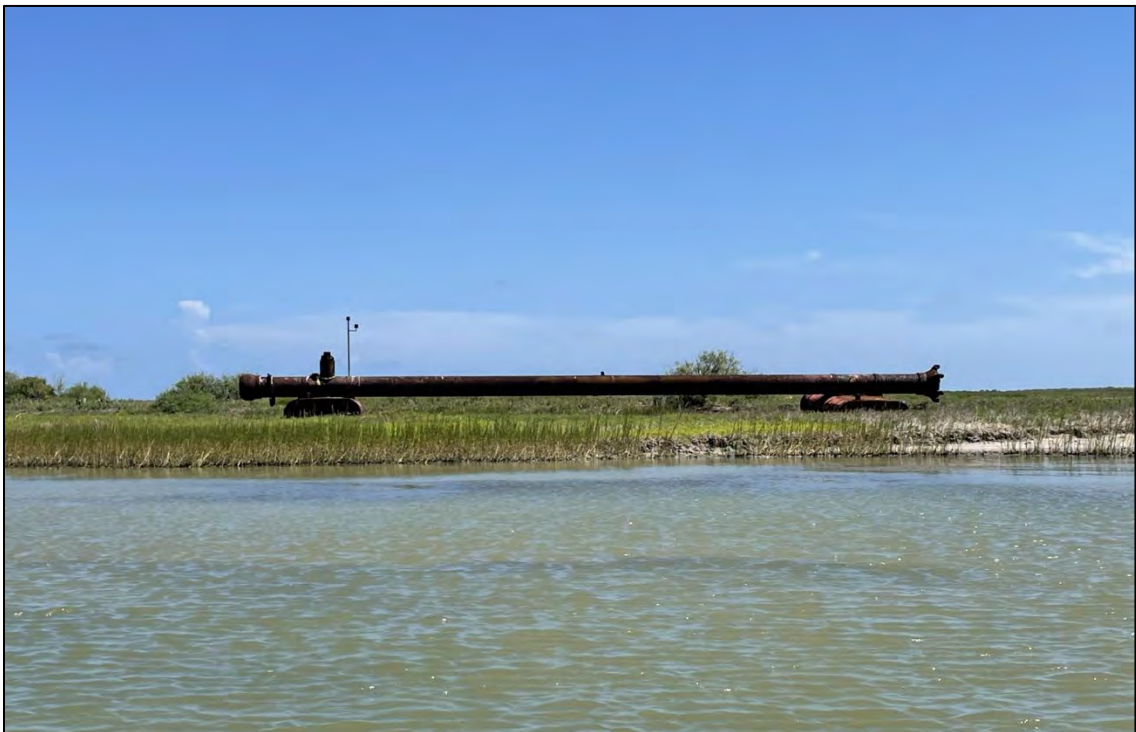
Photo 1. Abandoned dredge pipe located on Matagorda Island. The pipe is approximately 3 feet in diameter and 90 feet long.
