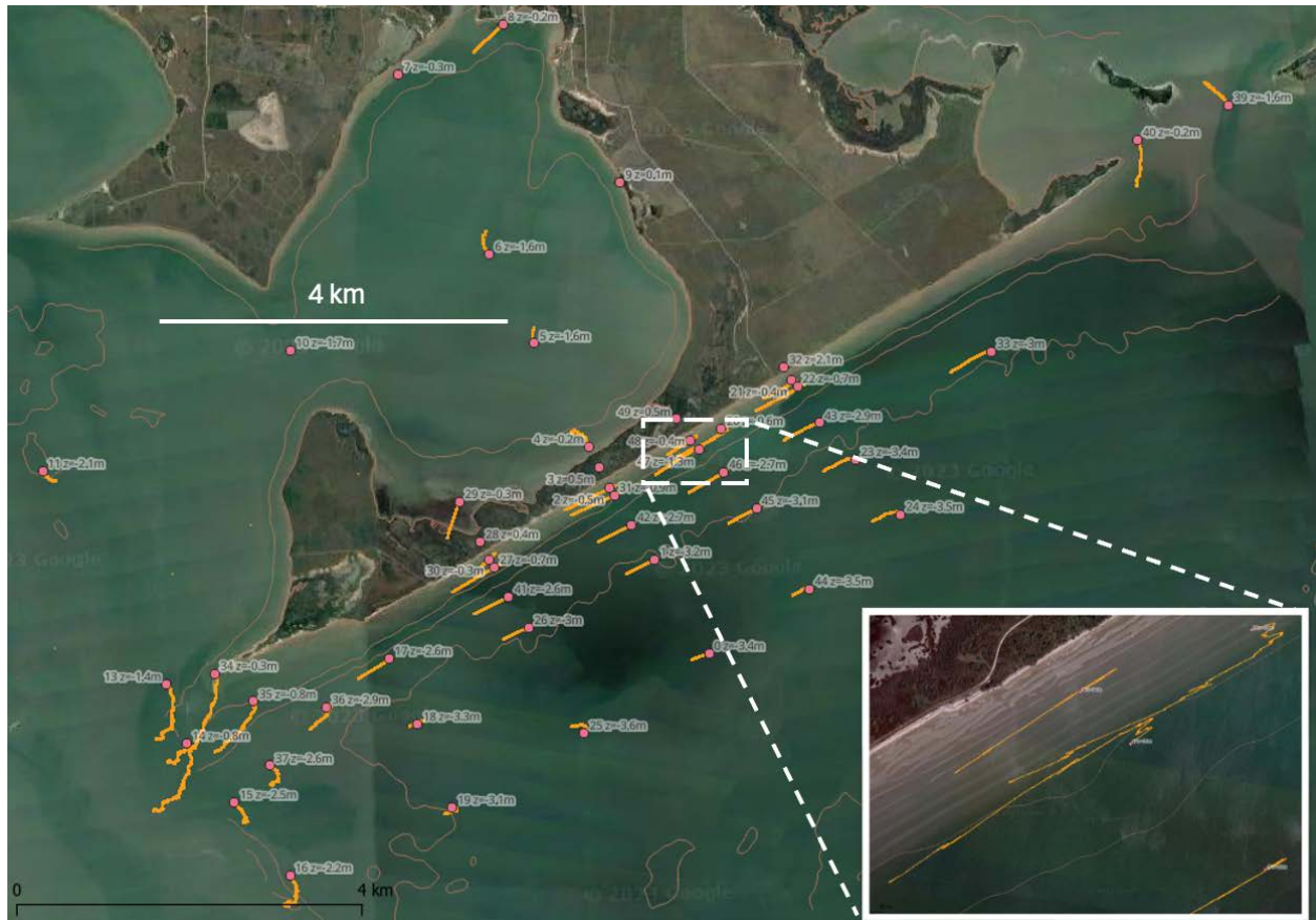
Fig. 18. An example of current flow tracks over time, generated by mapping flow velocities every hour iteratively. The origin is denoted by the small pink circles at the head of the orange line. The track around the tripod is shown in the zoom-in panel. The net tracks along the peninsula generally moved to the southwest due the most common wind and tidal conditions.
