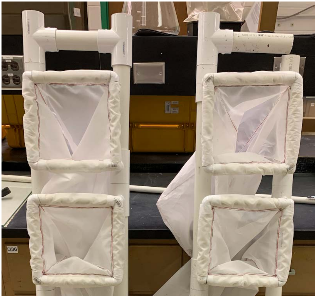
Figure 10. Two sediment streamer traps. Each trap had an upper and lower catchment trap.
