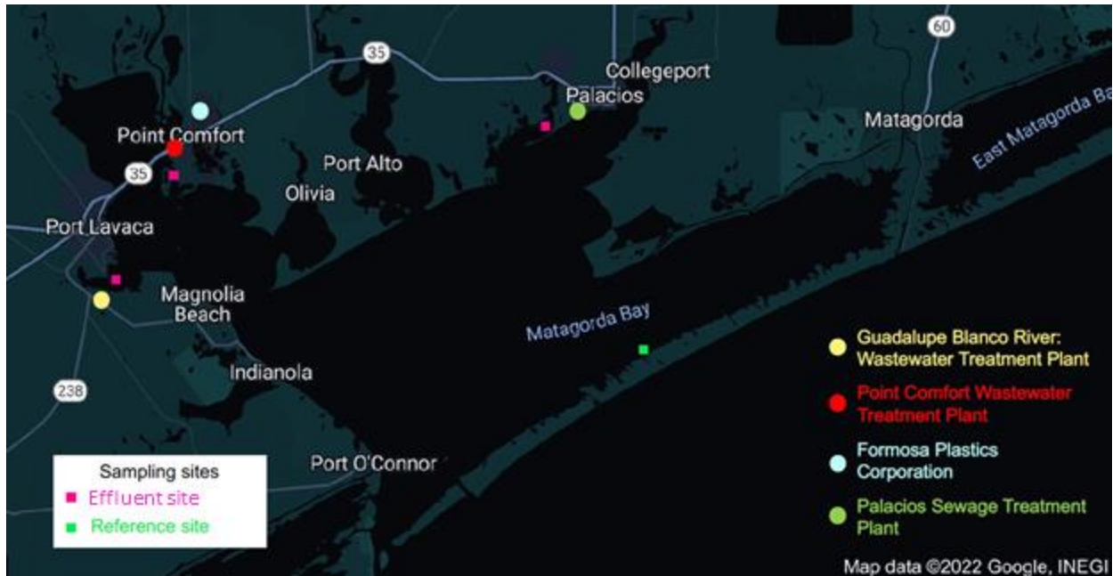
Figure 3: Proposed field sampling sites for the determination of lithium input into Matagorda Bay. All sites are associated with effluent inputs via wastewater treatment plants, while the reference site is intended as a non-effluent input site for the purposes of background values.
