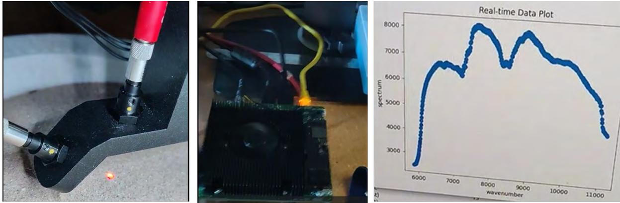
Figure 2. Screen video capture from lab testing of the rover spectrometer. Left image: spectrometer fixed on the rover arm. Middle image: rover computer unit. Right image: example of the continuous spectra measurements from the computer monitor.
