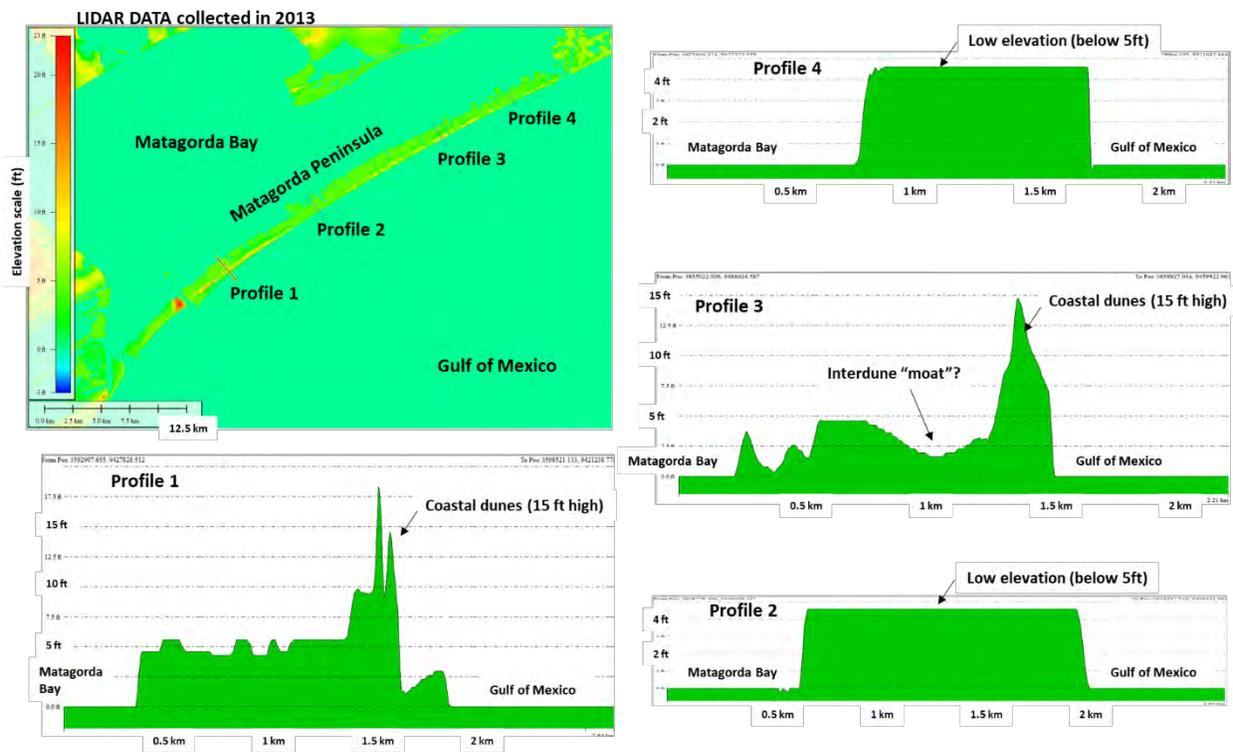
Figure 4. Matagorda Peninsula LIDAR map with the elevation profiles across the peninsula at different locations. Note the peninsula width is between 1 and 2 km, and the elevation varies at some locations less than 5 ft, and in other places it is 15 ft high.
