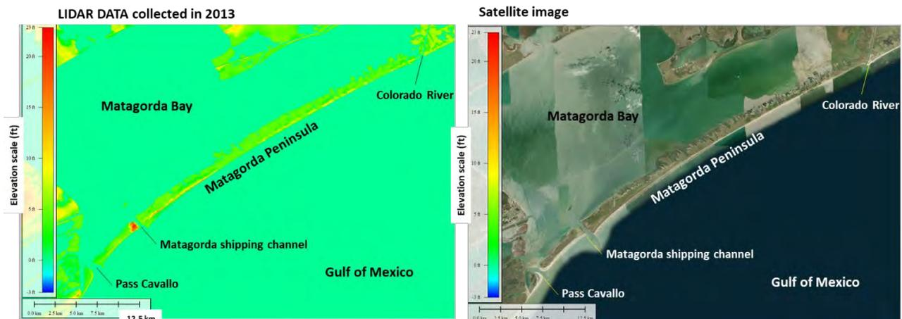
Figure 3. Matagorda Peninsula elevation and image. On the left: digital elevation model (DEM) from LIDAR data collected in 2013. On the right: satellite composite image.
