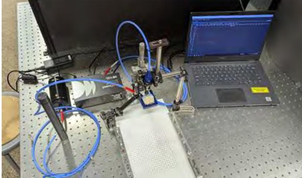
Figure 1: Fiber-coupled near-IR spectrometer for microplastic detection and classification.
