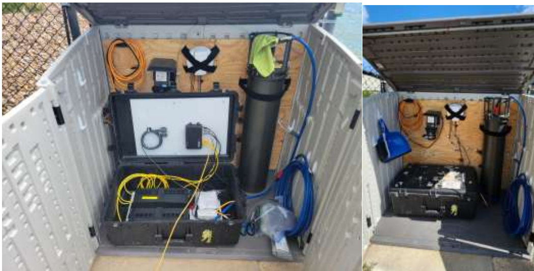
Figure 2. Deployment set up of IFCB175 and supporting equipment at TPWD Port O'Connor.
