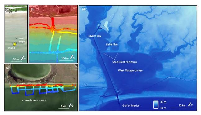
(a) The sensor tripod (yellow star) and sand traps were located 150 to 180 m offshore in West Matagorda Bay. (b-c) The topo-bathymetric point dataset for the immediate study area surrounding the tripod (colored dots), with 1 km long cross-shore transect (dotted white line), and (d) bathymetric dataset of the wider region, used for modeling purposes.
