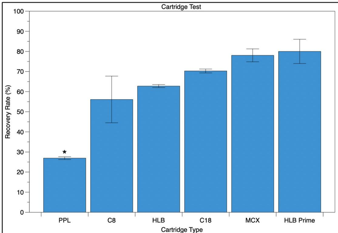
**Figure 8.** Recovery rate according to cartridge type.
